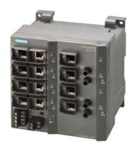
SCALANCE X212-2, managed IE switch, 12x 10/100 Mbit/s RJ45 ports, 2x 100 Mbit/s multimode BFOC, LED diagnostics, error-signaling contact with set pushbutton, redundant power supply, PROFINET IO device, network management, redundancy manager integrated, incl. electron. manual on CD-ROM, C-PLUG optional.
