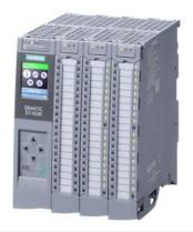
SIMATIC S7-1500 Compact CPU CPU 1512C-1 PN, central processing unit with working memory 250 KB for program and 1 MB for data, 32 digital inputs, 32 digital outputs, 5 analog inputs, 2 analog outputs, 6 high speed counters, 4 high speed outputs for PTO/PWM/frequency output 1. interface: PROFINET IRT with 2 port switch, 48 NS bit-performance, incl. front connector push-in, SIMATIC memory card necessary
