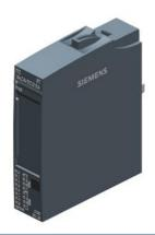
SIMATIC ET 200SP, Digital output module, DQ 16x 24V DC/0,5A Standard, Source output (PNP,P-switching) Packing unit: 1 piece, fits to BU-type A0, Colour Code CC00, substitute value output, module diagnostics for: short-circuit to L+ and ground, wire break, supply voltage
