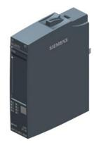
SIMATIC ET 200SP, Digital input module, DI 8x 24V DC Standard, type 3 (IEC 61131), sink input, (PNP, P-reading), Packing unit: 1 piece, fits to BU-type A0, Colour Code CC01, input delay time 0,05..20ms, module diagnostics for: short-circuit of sensor supply, wire break, supply voltage
