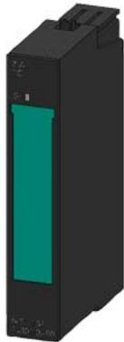
\*\*\* Spare part \*\*\* SIMATIC DP, Electronics module for ET 200S, 2 AI TC standard; 15 mm width, 15 bit+sign +/-80 mV; Characteristic linearization for thermocouples of the types: B, E, J, K, L, N, R, S, T Cycle time 65 ms/channel with SF LED (group fault)
